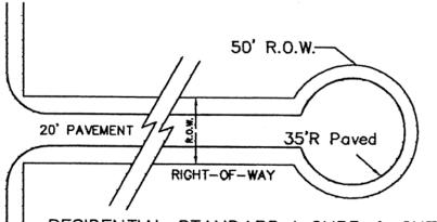
RESIDENTIAL STANDARD I CURB & GUTTER SECTION 50 FT. CUL-DE-SAC, R.O.W., 35 FT. PAVED RADIUS
