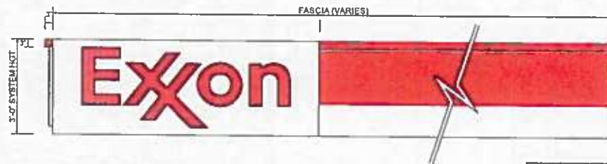
THREE (3) LED ILLUMINATED CANOPY "EYEBROW" RAIL SYSTEM.
