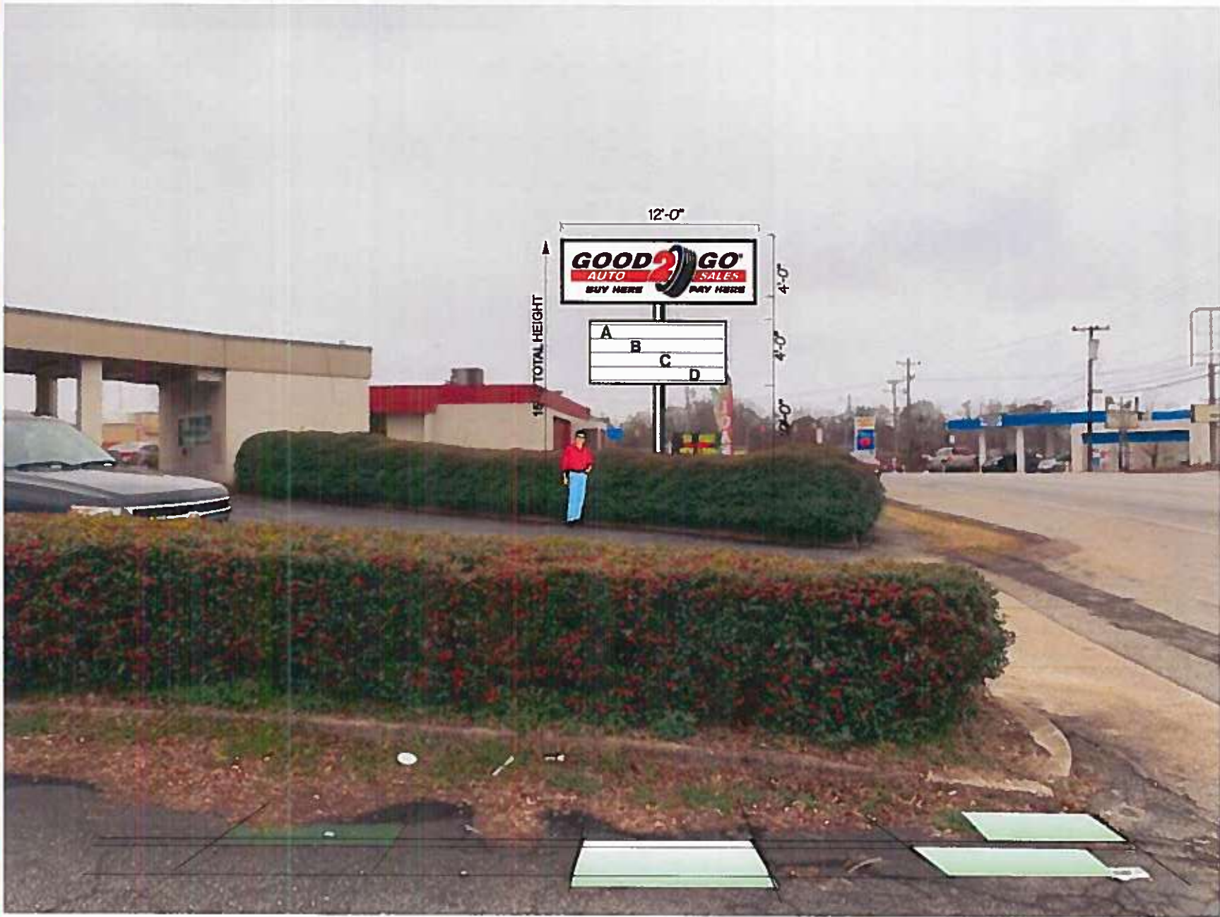
Front Elevation double face illuminated sign
