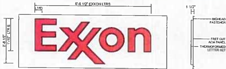
THREE (3) 2D EXXON ACM LOGO BOX CANOPY SIGNS. THERMOFORMED LETTERSET MOUNTED TO ACM BOX. BOXES TO BE INTERNALLY ILLUMINATED W/ WHITE LEDS.
