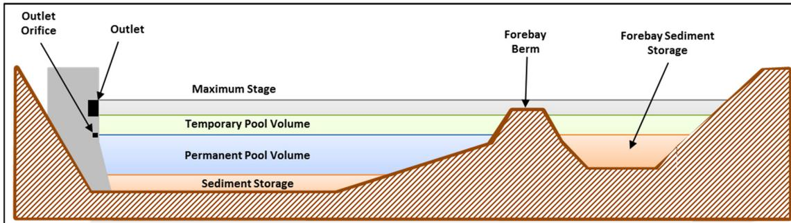
**Figure 2: Plan View of a Wet Detention Basin**
