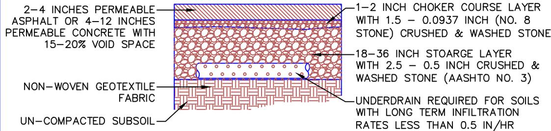
**POROUS ASPHALT & CONCRETE DETAIL**
